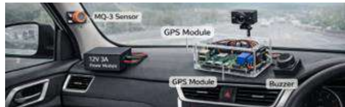
Fig. 6: SafeWheels system installed inside a vehicle.
